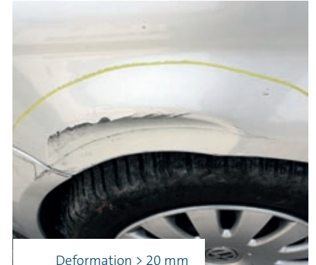
Deformation &gt; 20 mm
